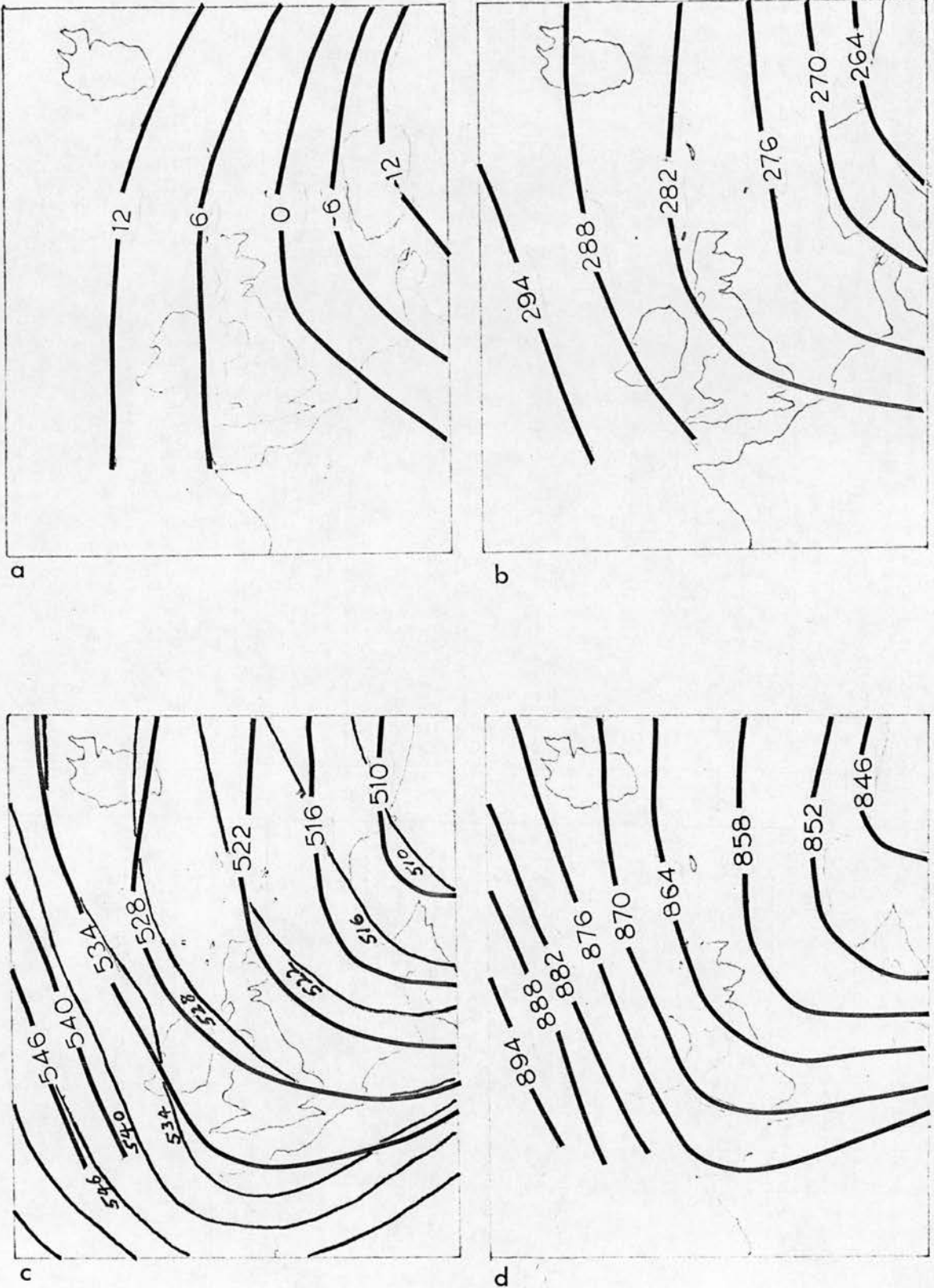
Figure 5.12 Objectively analysed surfaces, 2nd January 1965, 00Z. (a) 1000 mb (b) 700 mb (c) 500 mb, thin lines from U.K. Daily Aerological Report 500 mb analysis (d) 300 mb (Contours in decametres).
