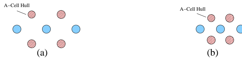
Figure 4.9: The pattern formed by intermixed A-Cells. (a) Low heterotypic adhesion. (b) Higher heterotypic adhesion pulling the A-Cells closer together.
