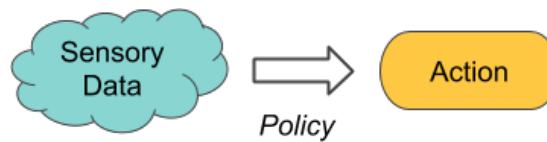
Figure 8: A policy is a direct mapping from sensory data to an action.
