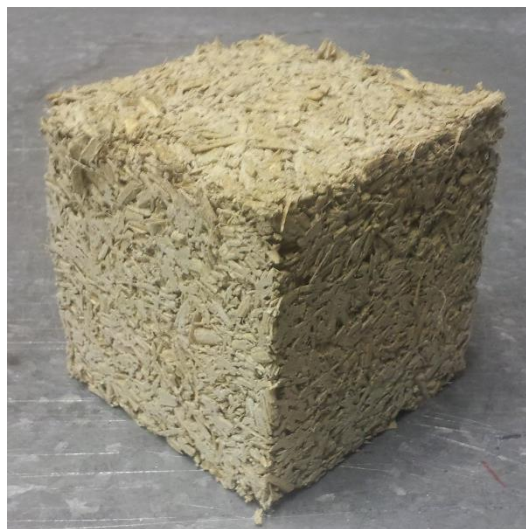
Figure 4.2 – Rigid cast cube of completed hemp-lime insulation with dimensions 100 by 100 by 100mm.
