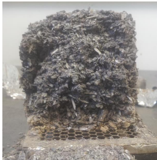
Figure 5.17 – Remnants of a PCM hemp-lime specimen tested at 8\text{kW}\cdot\text{m}^{-2} . Partial collapse of the sample occurred upon removal of the foil and insulation.
