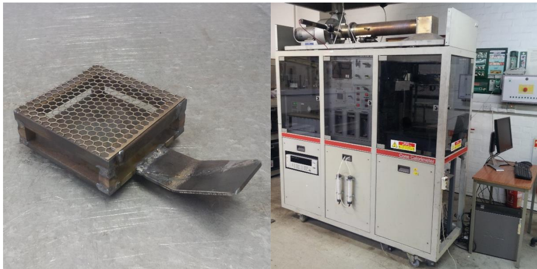
Figure 4.4 – (a) Porous sample holder used for testing (b) Cone calorimeter at the University of Edinburgh.
