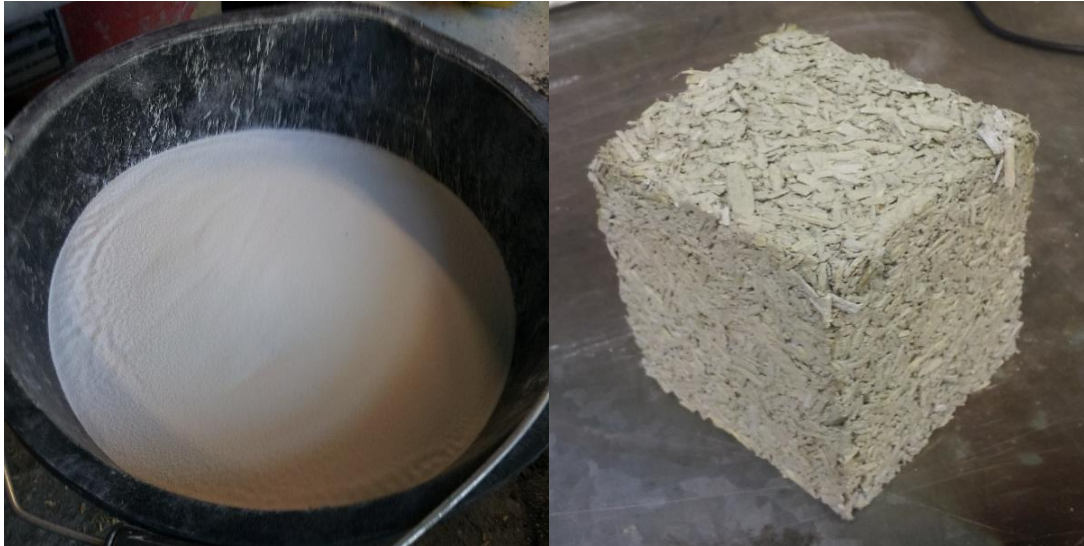
Figure 5.1 – Photographs of (a) raw microencapsulated PCMs which have a powder-like appearance and (b) completed cube of PCM enhanced hemp-lime insulation (100mm by 100mm and 100mm tall).
