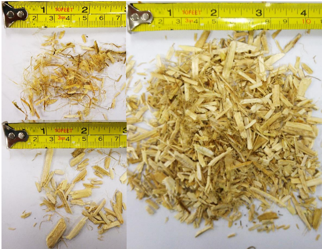
Figure 4.1 – Hemp shivs and fibres used in the casting process. Top left: woody pulp which makes up only a small portion, bottom left: the main shivs and fibres (cores) which make up the majority of the mass, right: general overview.
