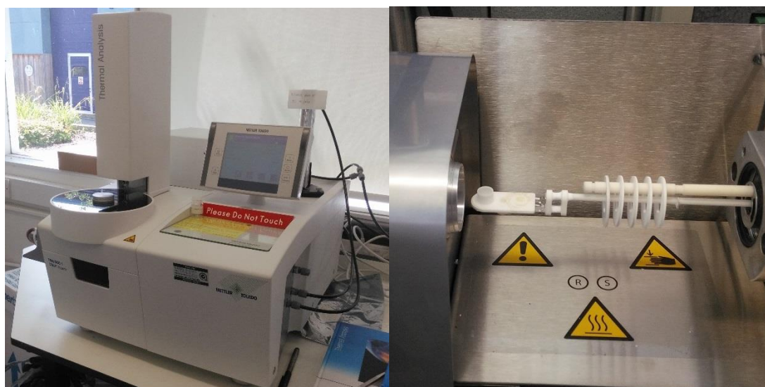
Figure 3.5 – Mettler Toledo TGA/DSC 1 at the University of Edinburgh. (a) Overall view of apparatus (b) view of weighing arm. The furnace is visible to the left of the photo, and the sample crucible is already placed on the arm.
