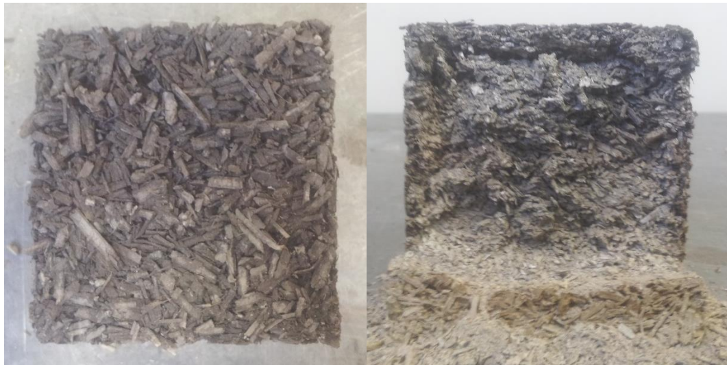
Figure 4.10 – Remains of hemp-lime insulation tested at 8\text{kW}\cdot\text{m}^{-2} . (a) View of top surface (b) splice sawed through sample.
