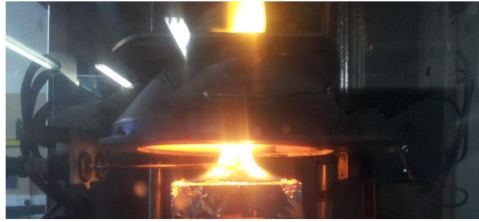
Figure 6.2 – Photograph of PCM plasterboard exposed to 80\text{kW}\cdot\text{m}^{-2} for illustrative purposes.
