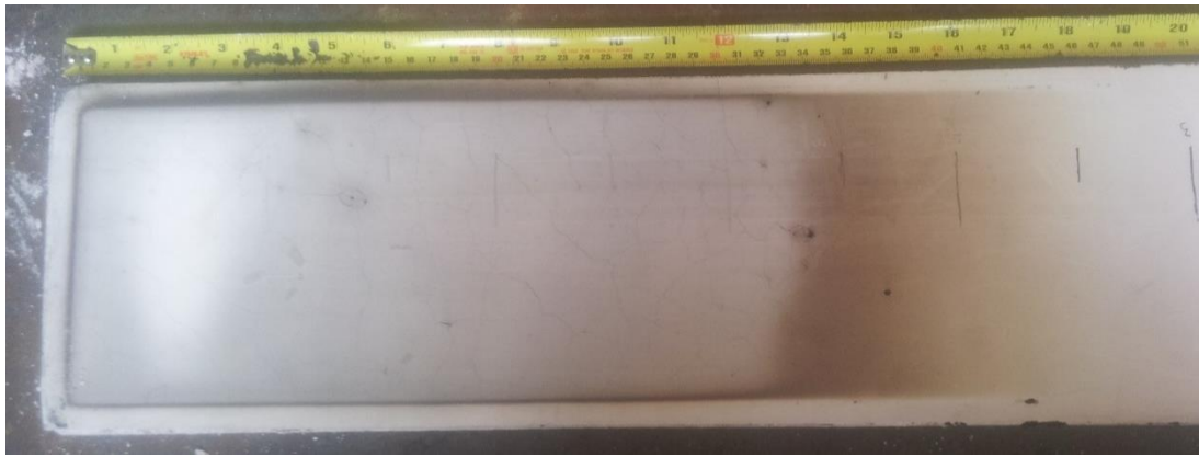
Figure 7.23 - Sample 2 following testing for approximately 12 minutes of thermal exposure.
