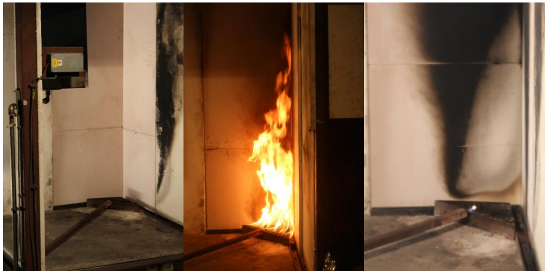
Figure 7.24 - SBI test setup: (a) Burners and PCM plasterboard in corner with joint visible (b) main burner during test (c) bottom section after testing.
