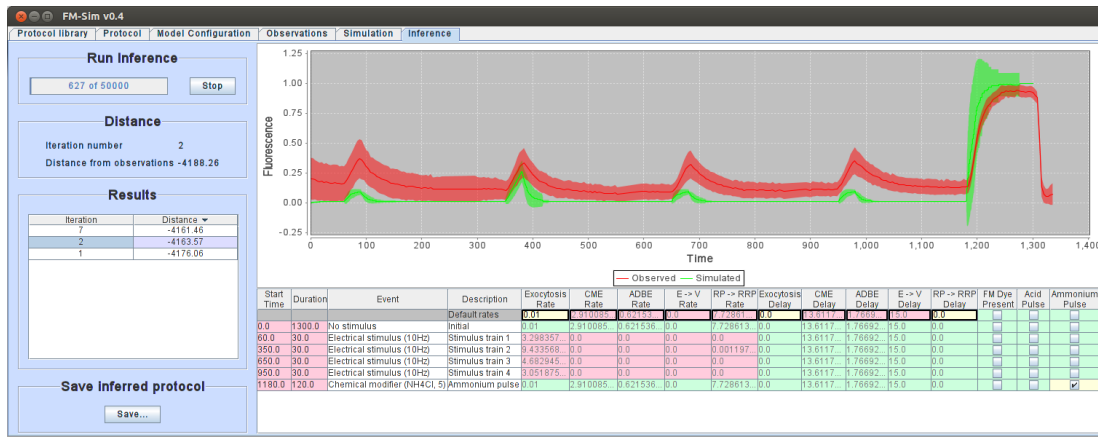
Figure 8.3: Example parameter inference of a defined protocol, the parameter values in red are inferred from observed experimental data. The graph shows a sample simulation using these parameter values (green) compared against the supplied experimental data (red).
