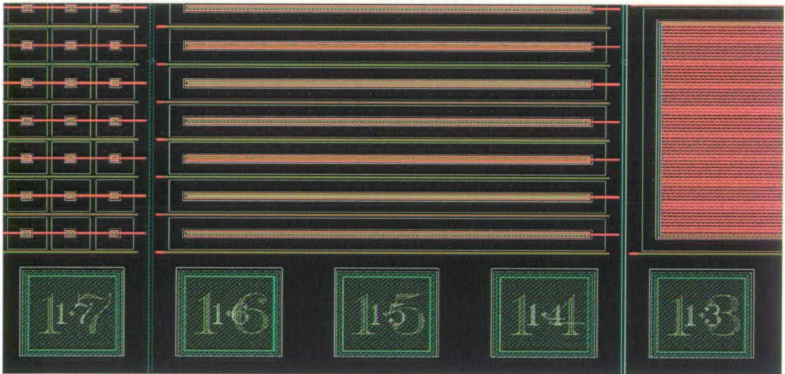
Close-up of the junction diode test-structure, on the left one can see the dotted structures, in the middle the stripe and on the left the planes.
