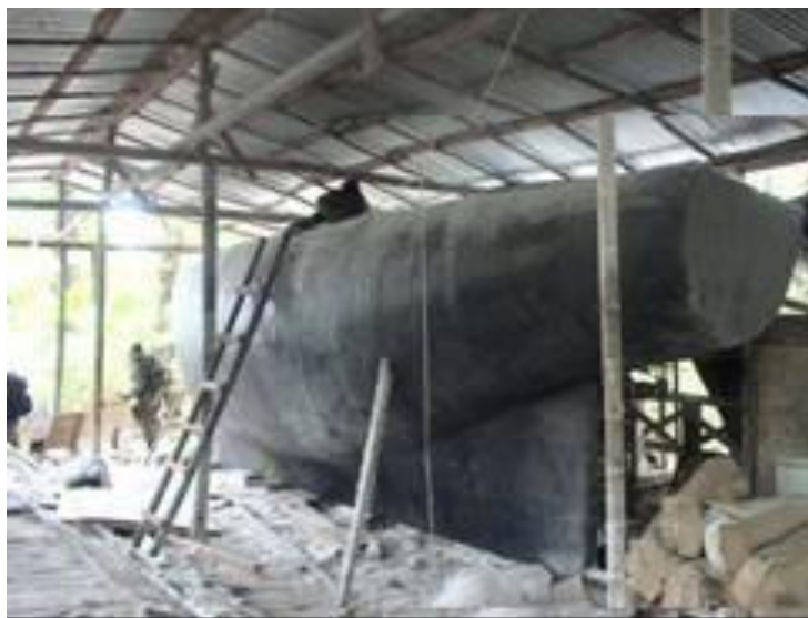
Figure 32. Semisubmersible in the making. Source: unk, Provided to author by an ex intelligence detective.
