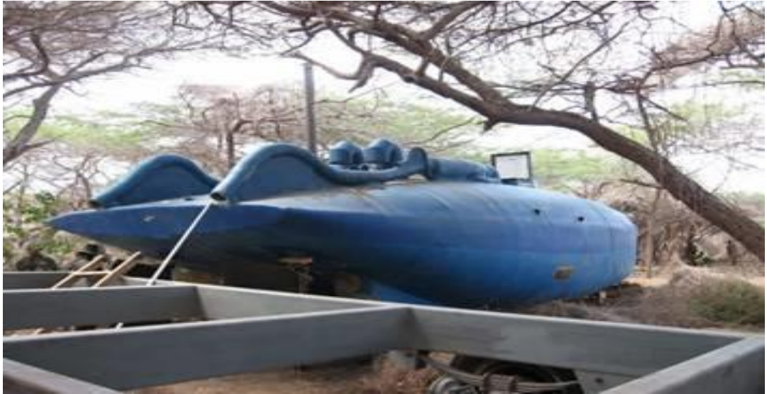
Figure 45. Steel hull semisubmersible, La Guajira. Source: Colombian Antinarcotics Police.
