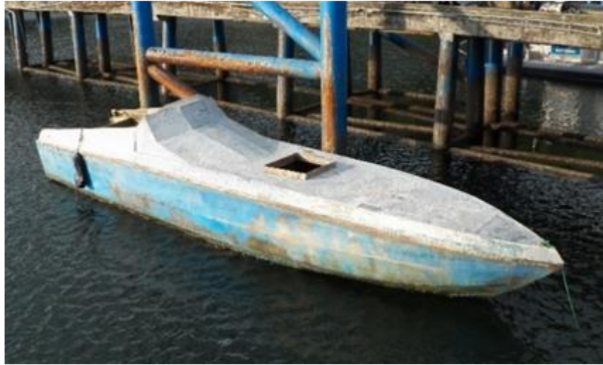
Figure 11. Makeshift Go-fast boat. Source: Author
