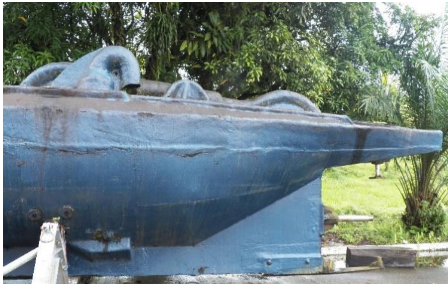
Figure 39. 'Goose neck' exhausts in fibreglass. Source: Author.
