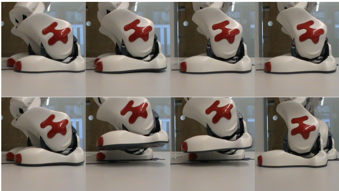
Figure 5.7: Detail of a left foot swing. Top row : the original trajectory that provides minimal foot clearance (approx. 2cm on apex). Bottom row : adding a obstacle close to the original trajectory pushes the optimization to higher stepping trajectories (here approx. 5cm on apex).
