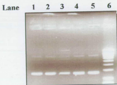
Figure 2.2: UV illuminated agarose gel. Lanes 1,2,4,5; pDSb 2 containing DNA coding sequence for flavocytochrome b 2 containing the N42C:K324C mutation (samples 1-4), Lane 3; pDSb 2 containing DNA coding sequence for wild-type flavocytochrome b 2 , Lane 6; 1 kb marker (GIBCO).
