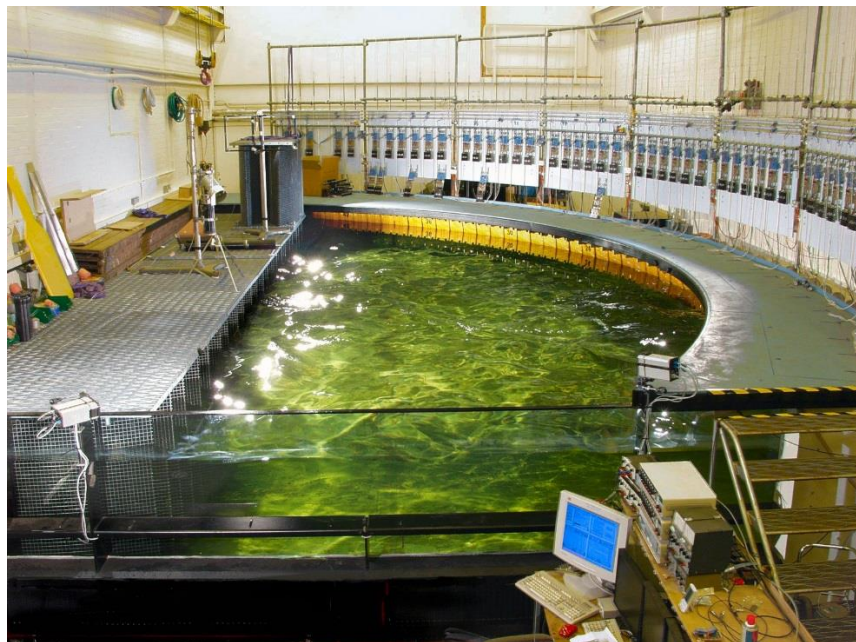
Figure 2.2: The curve flow testing tank in the Edinburgh University. The sea state curve tank can generate wave from different direction and can be used for wave condition exploring. It can also be used in ocean structure testing and analyse its interaction with waves.
