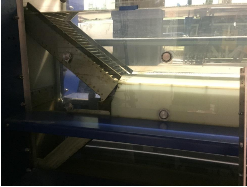
Figure 2.6: Vanes in the Flume. The sub-vane is used in the tank for flow direction restriction. Steady uniform flow can be created in the flume without strong interaction with water surface near input flow.
