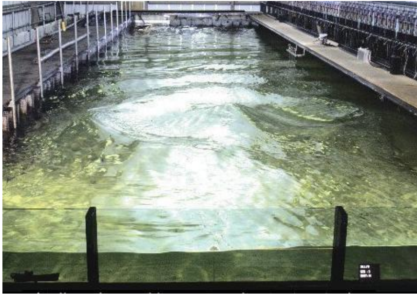
Figure 2.1: Wide tank that ever in service in the Edinburgh University. It was constructed for in wave condition simulation in ocean and structure testing. It has been teared down after working 24 years.
