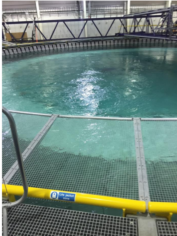
Figure 6. 3: Uniform flow generated in the circular basin. The velocity of the flow is 0.8\text{ms}^{-1} and the direction is changed by combined controlling of impellers as shows in chapter 2.
