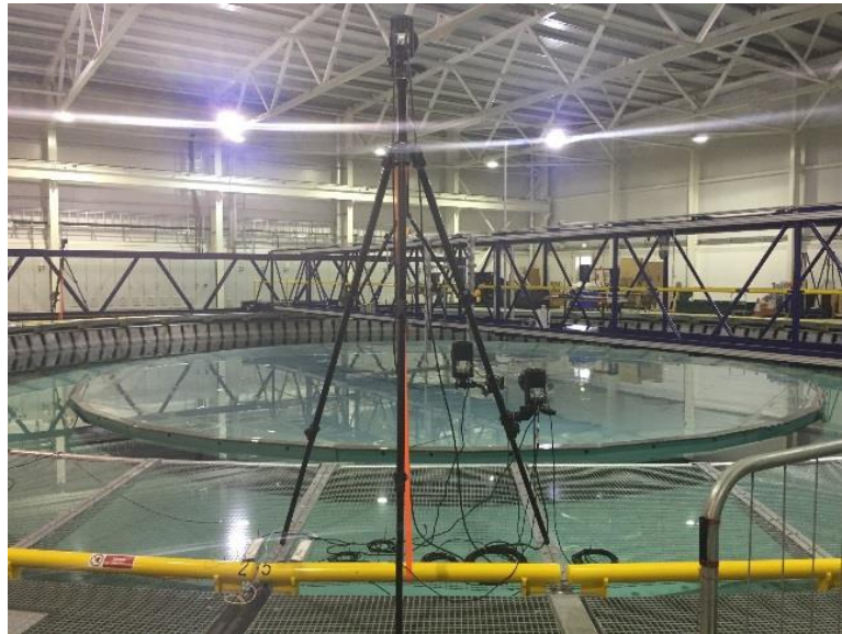
Figure 2.4: Section of the FloWave Facility. Steady flow is generated by the impellers that installed underneath the testing floor along the perimeter.
