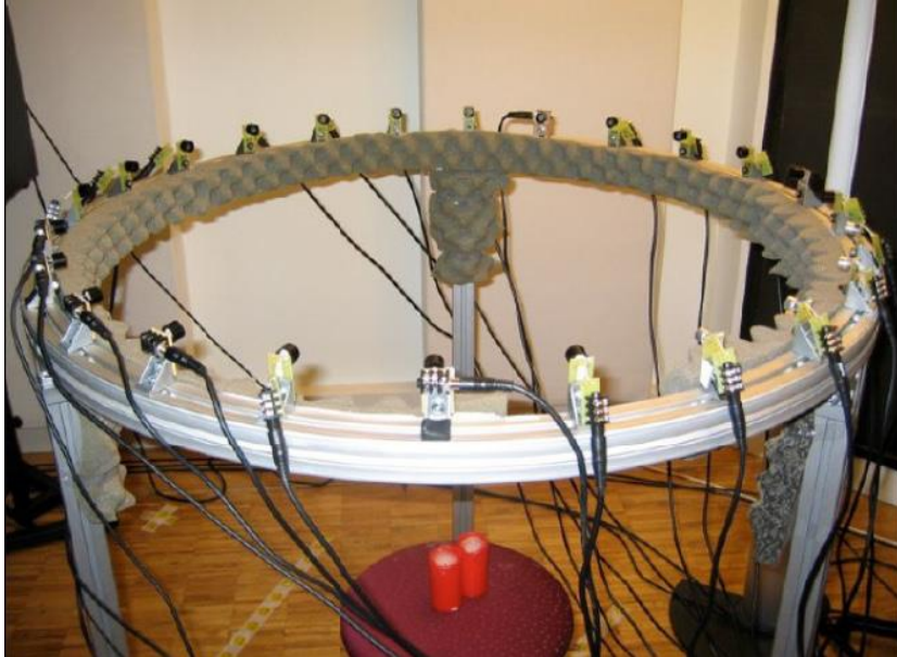
Figure 2.13: Air temperature sensing system using acoustic tomography method [104]. The sensing system consists of 12 sound transmitter and 12 receivers. The sensors are installed along the circumference of 1m radius circular ring. A heat source is placed under the sensing network for air temperature heating.
