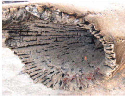
Figure 1.5: Cavity left by smoldering inside a log (Costa and Sandberg 2004, reproduced with permission).
