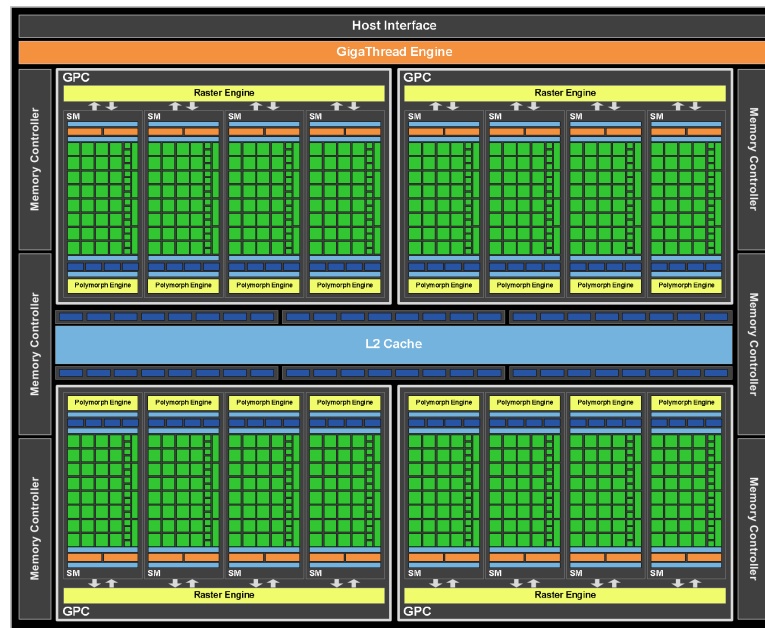
Figure 2.4: Schematic representation of the Fermi GF100 architecture. Taken from [100]
