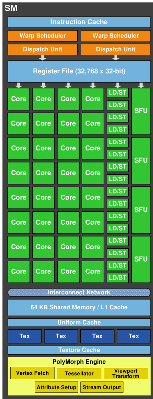
(a) Schematic representation of a Streaming Multiprocessor.
