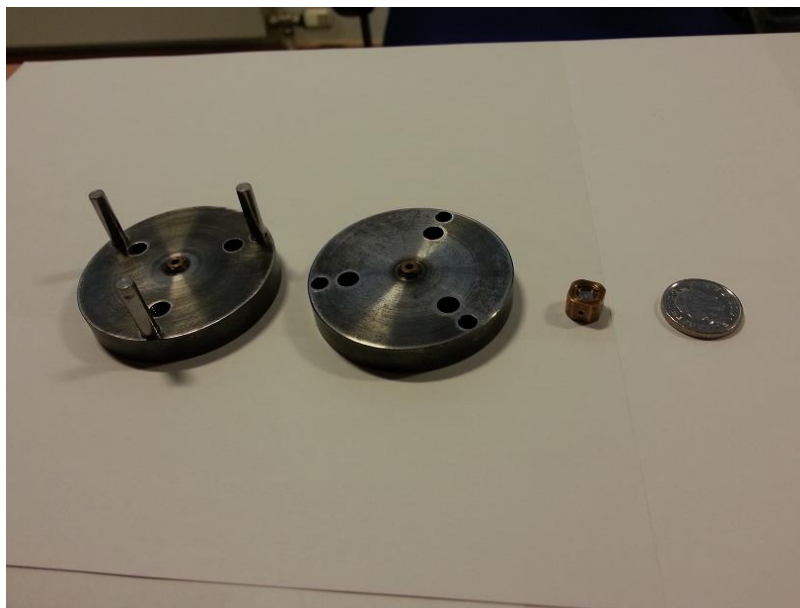
Figure 3.2: Clamps used for applying pressure in the turnbuckle cell
