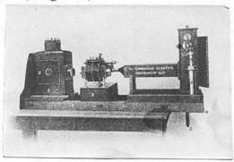
By means of a micrometer screw, the tension of the string may be altered so as to vary the sensitiveness of the galvanometer. The string is in connection with two terminals to which the wires are attached which convey the current generated in the patient to the galvanometer. Figure 4 represents a photograph of the galvanometer.
