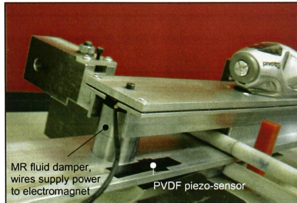
Figure 5-4: Concept verification, with MR fluid damping of (aluminium) ski-like fore-body structure on ski simulator moment arms
