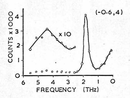
Preliminary results for the dispersion relations of DKDP at  $300^{\circ}$ K as measured on the small DKDP crystal. The solid lines represent a least squares fit to the acoustic modes only using a simple lattice dynamical model described in chapter 3.
