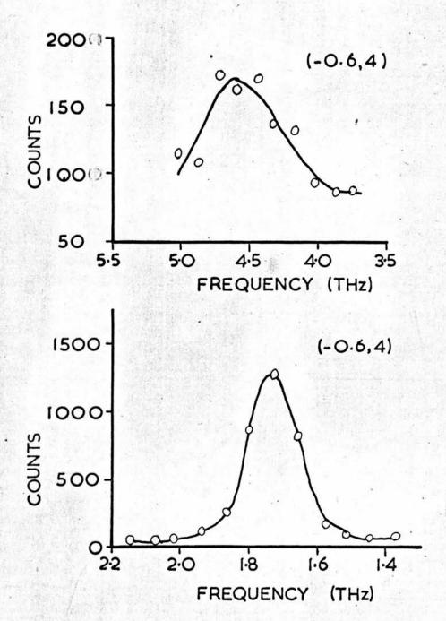
Phonon dispersion relations of DKDP at 300°K. The measured values and the errors are given in table 2.2. The solid lines represent a best least squares fit to the data as described in chapter 3.
