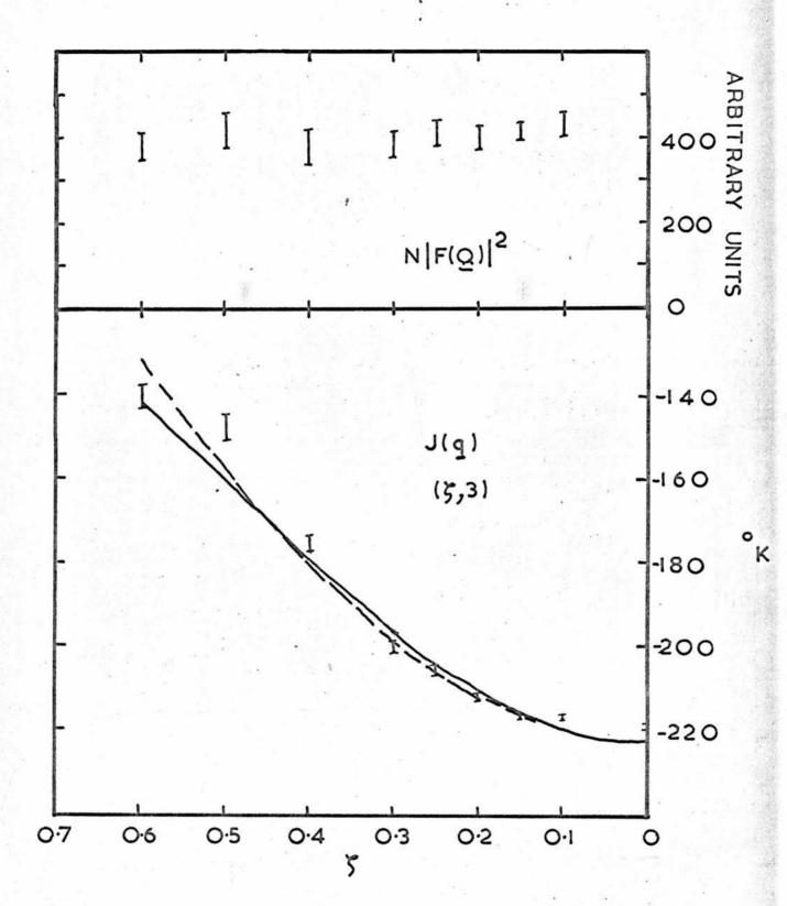
The interaction  $I(\mathbf{q})$  and structure factor squared  $N | \mathbf{F}(\mathbf{Q})|^2$  along the lines  $(2,4,\eta)$ ,  $(2,6,\eta)$ ,  $(2,8,\eta)$ ,  $(2,9,\eta)$  and  $(3,0,\eta)$ . The solid curves for  $I(\mathbf{q})$  use only nearest neighbour interactions and a separate Coulomb interaction,  $V_{\mathbf{c}}$ , for each line, while the dotted curves use next nearest neighbour interactions and one value for the Coulomb interaction.
