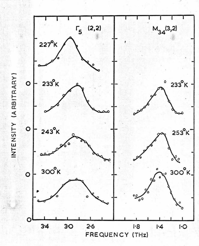
Constant energy scans with zero energy transfer along the line (5, 3.2) near the reciprocal lattice point (3, 3). The monitor count was  $10^6$  neutrons. The peak at 5 = 2.4 may be due to 5th order Bragg scattering. The shape of the scattering indicates that it is not incoherent and the temperature dependence shows that it is associated with the ferroelectric transition. The nearest reciprocal lattice points along the line (5, 3) are (1, 3) and (5, 3).
