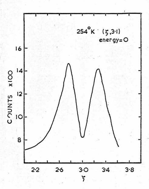
Distribution of the quasielastic critical scattering in the ( $\lesssim$ ,  $\chi$ ) plane around the reciprocal lattice point (3, 3). The contours are not equally spaced as can be seen by comparing figure 2.8.
