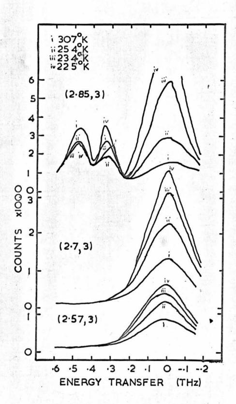
The intensity of the quasielastic critical scattering along the line (5,3). The width of the Bragg peak is shown in the left hand side of the figure. The Bragg peak has been subtracted from the distributions shown on the right hand side, which illustrate the temperature dependence of the critical scattering.
