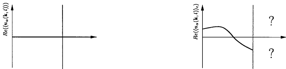
Figure 2.1: Schematic illustration of the way in which we select members of the biased subensemble, and the results we would expect if we perform an ensemble average over each of these sets of realizations. The dotted lines indicate the limits of the range u^- \pm \xi . Note that since \langle u \rangle = 0 , the average lies along the ordinate in the case of the full ensemble.
