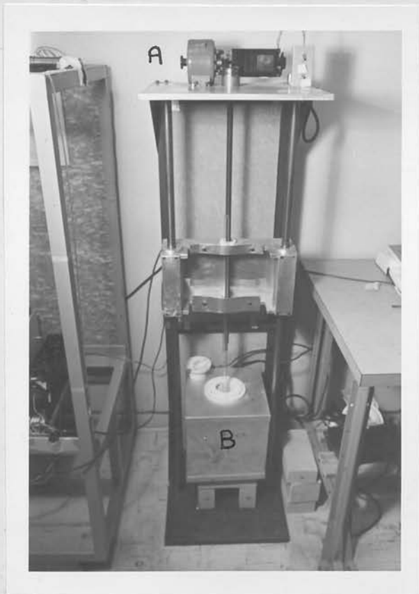
(b) Kanthal furnace and puller. A. Drive system. B. Furnace.
