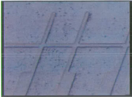
FIGURE 2. 16 \mu\text{m} segment of SCCDRM fabricated in bulk silicon on 200 mm wafer.
