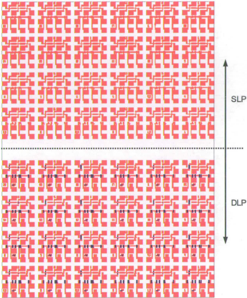
(a) Test chip design for evaluating both SLP and DLP patterning techniques
