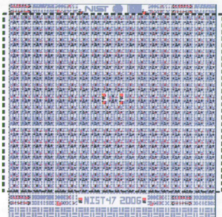
Figure 3.7: Layout of NIST 47 design; the test structure described is the 16 by 18 array of cells indicated.
