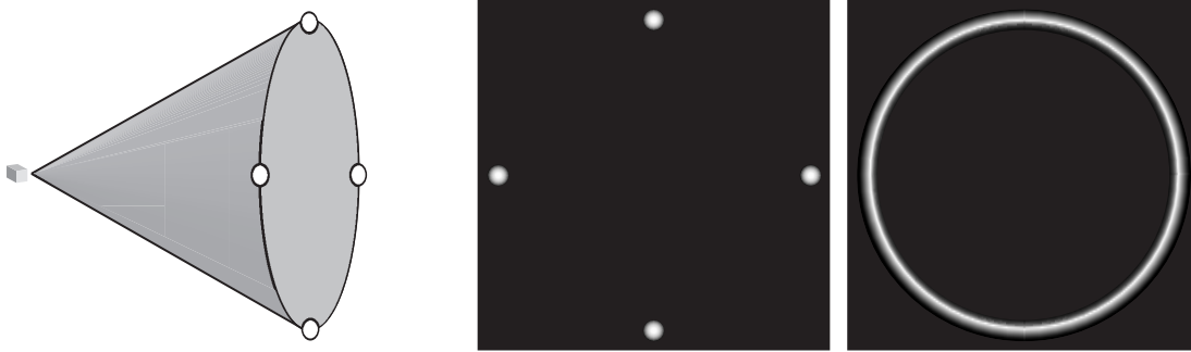
Figure 2.3: Diffraction of multiple reflections with identical d -spacing (left) leading to individual Bragg reflections for the single crystal case (centre), and Debye-Scherrer rings for the polycrystalline case (right).
