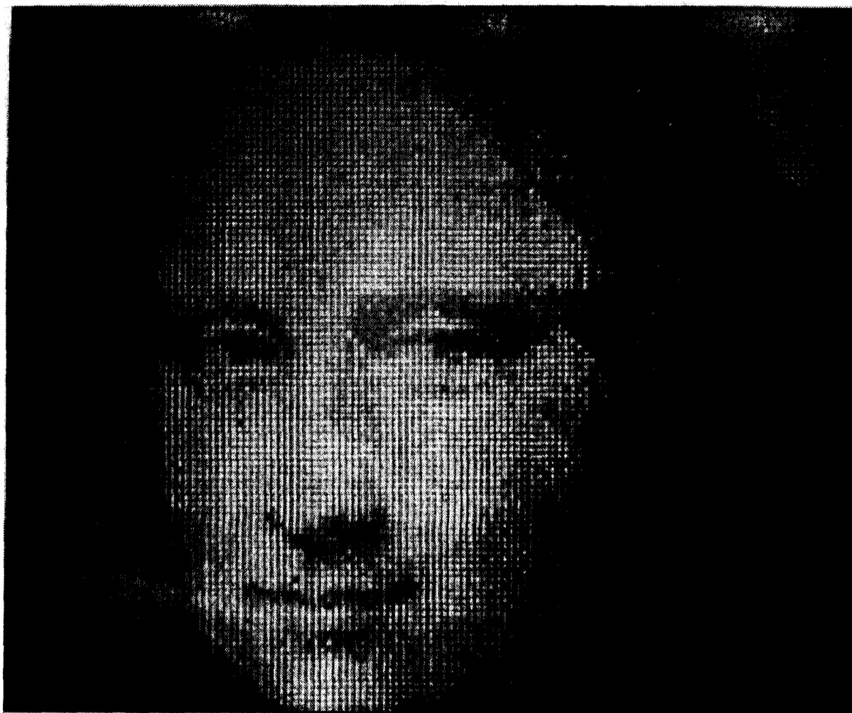
Figure 5–18: ‘Mona Lisa’ grey-scale test pattern on a section of an unplanarised SLM (8#2). Fifteen bit-planes are used to render the temporally multiplexed grey-scale. Because of an error in the driving software, this device was not properly charge balanced – note that a previous ‘triangle’ pattern is still partially visible.
