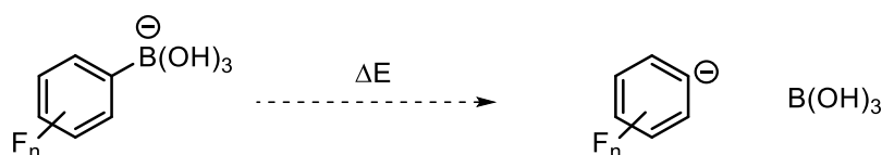
Scheme 4.3 Unimolecular fragmentation process used to in the quantum chemical calculations of the in intrinsic energy differences ( \Delta E ).
