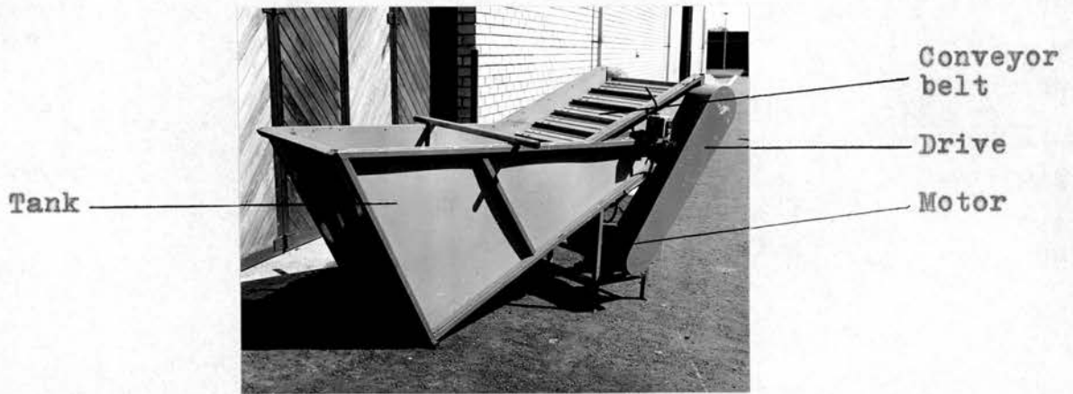
Plate 16. General view of prototype continuous disinfection tank.
