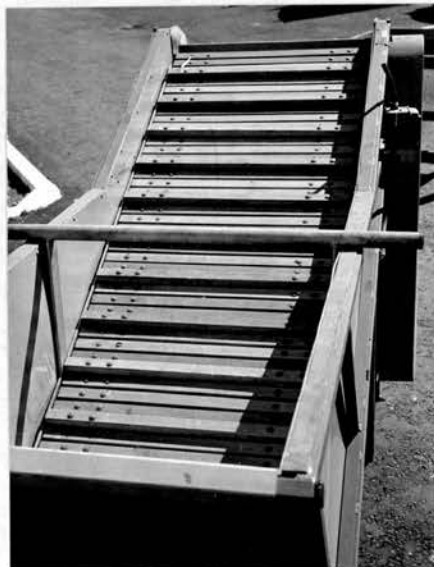
Plate 17. Detail of conveyor belt running from the base of the tank.
