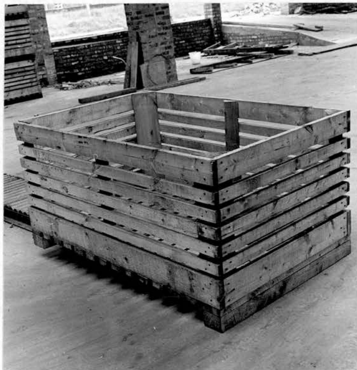
Plate 1. A 10 cwt. box as used for final drying of washed and disinfected seed tubers at the commercial plant.
