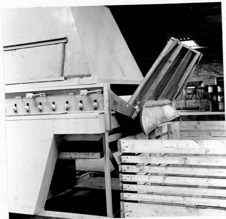
Plate 5. Part of a sponge roller drying table under a high capacity fan at the point where tubers enter the 10 cwt. boxes.
