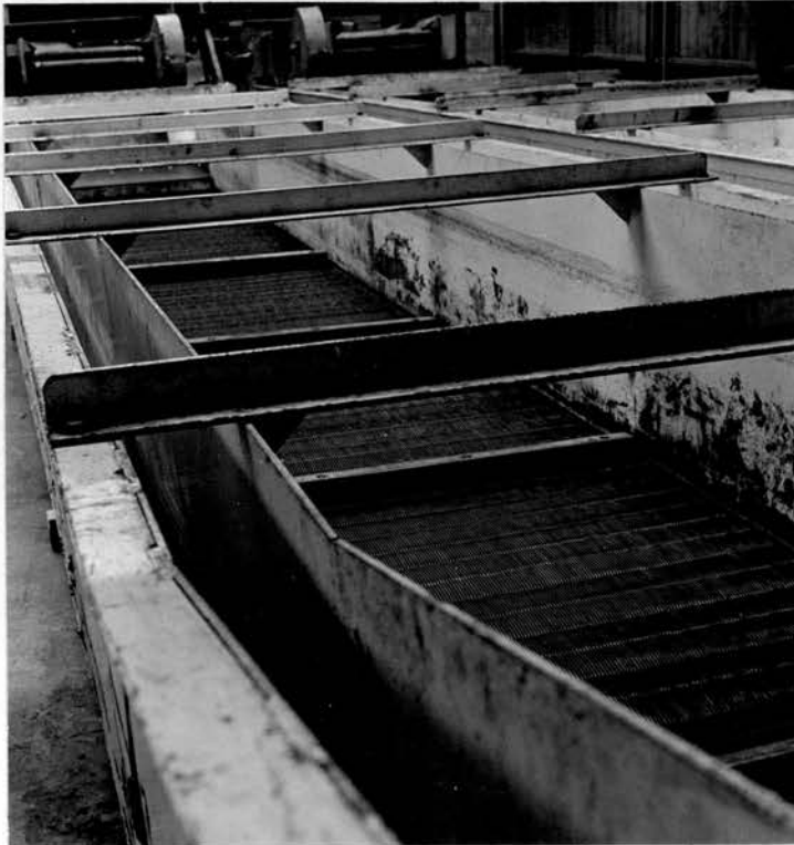
Plate 9. A disinfection tank showing the conveyor belt which moves tubers through the solution.
