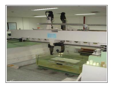
**Figure 4.3:** The physical modelling system for 2-D data acquisition in the laboratory. The base model is submerged in a water tank.
