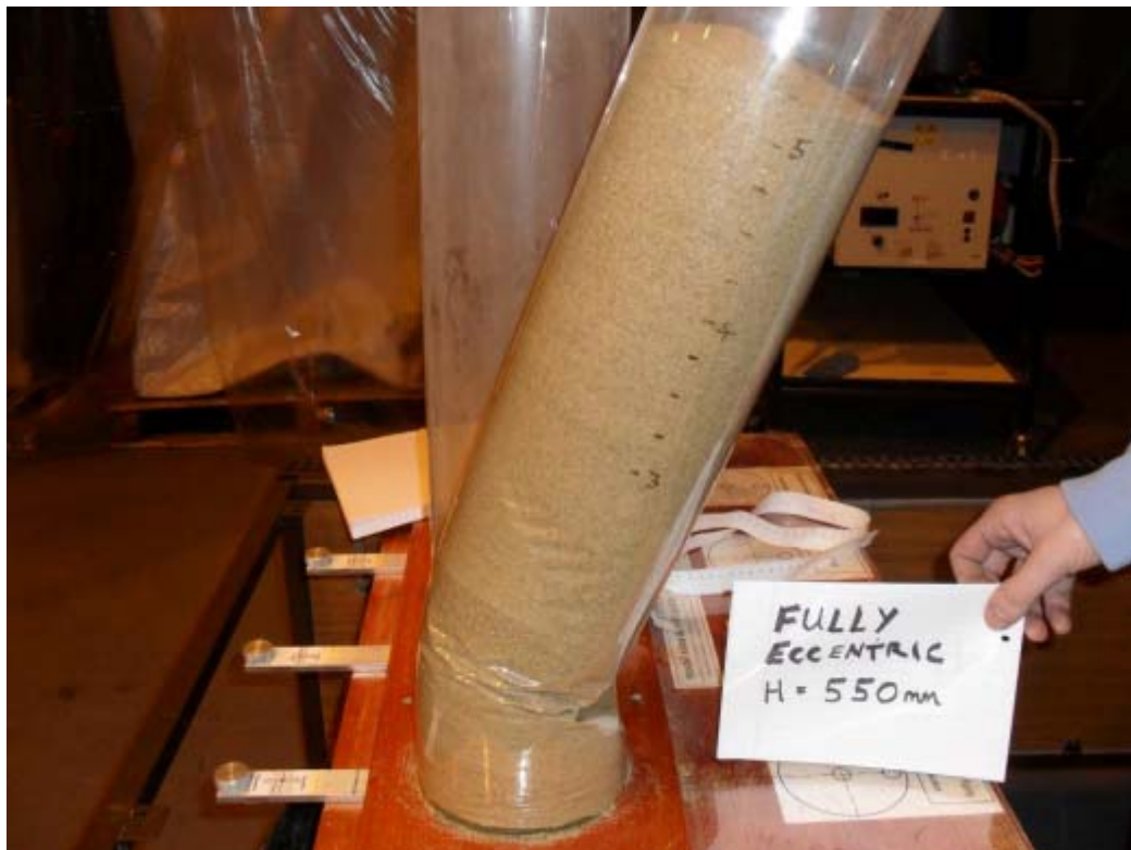
b) Global overturning collapse of a model silo under fully eccentric discharge (after Watson, 2010)
