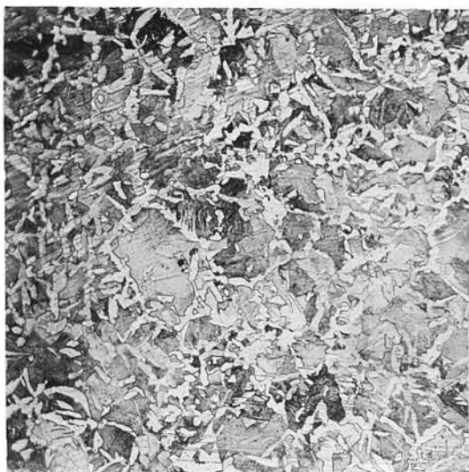
Fig. 11. Steel A. Austenised 900°C Reacted 8 min. at 680°C x 100.
