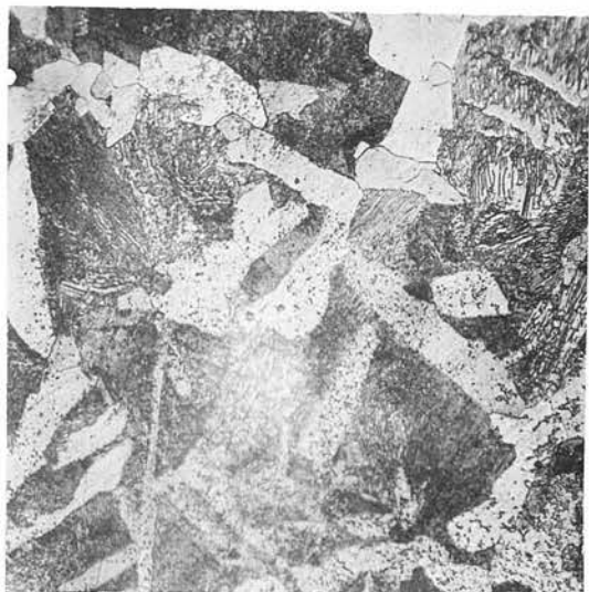
Fig. 12. Steel A. Austenised 900°C Reacted 8 min. at 680°C x 500.
