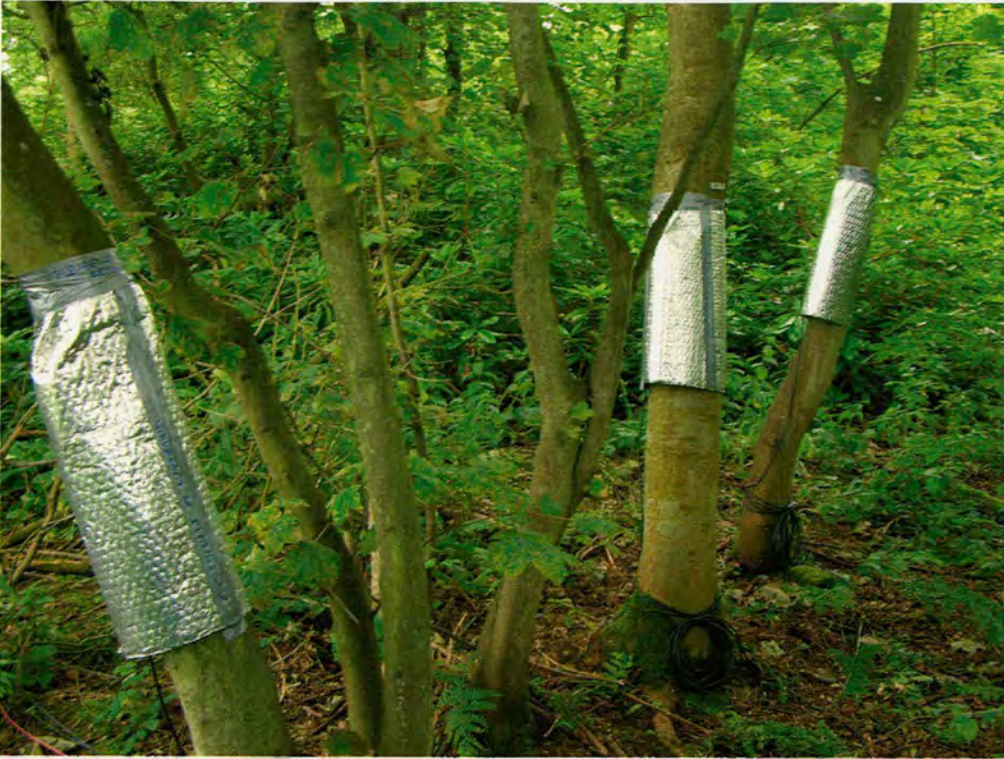
Plate 4.2: Insulation sheets were applied around the stem where sensors were installed to protect them from rainfall and convective heat losses.
