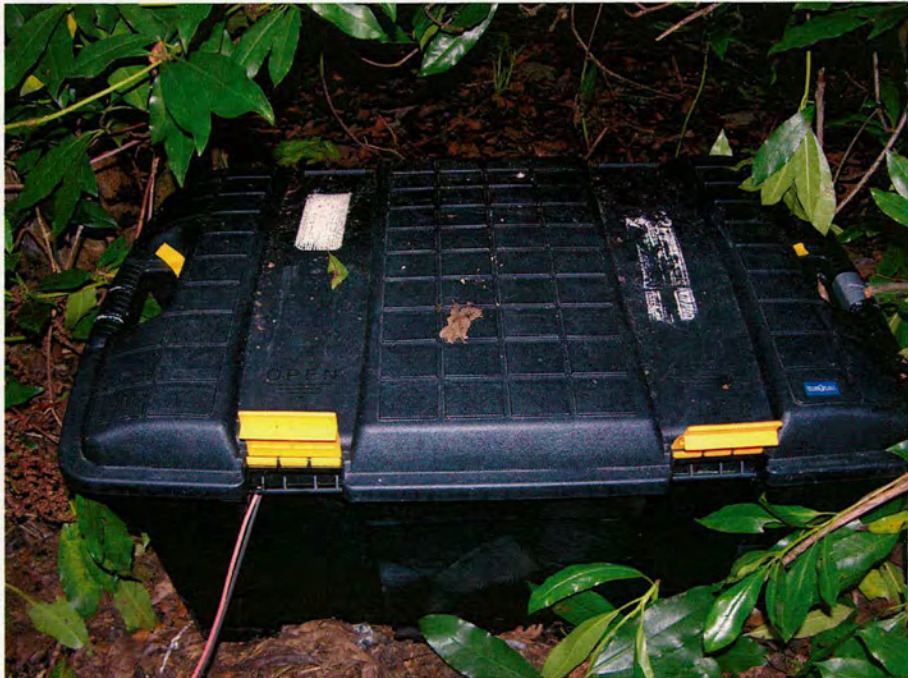
Plate 18 : Batteries to power the dataloggers and heating boxes were kept in this box to avoid exposure to rain etc.
