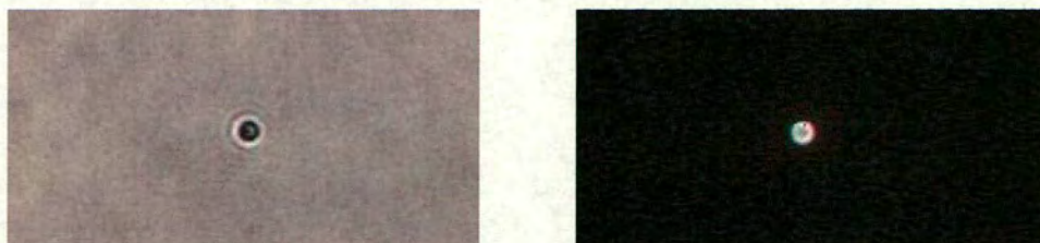
Figure 3.5: Brightfield (left) and fluorescence (right) images of the same trapped bead.
