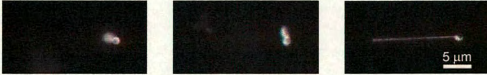
Figure 3.8: Fluorescence imaging of DNA: (left) and (centre) the DNA polymer at zero flow, (right) the DNA stretching when flow is introduced in the flow cell.
