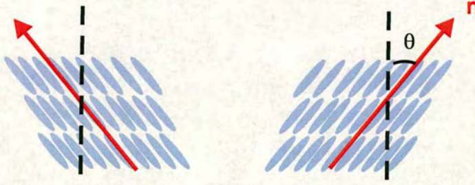
Figure 7.2: The switching of a FLC when opposite electric field is applied.
