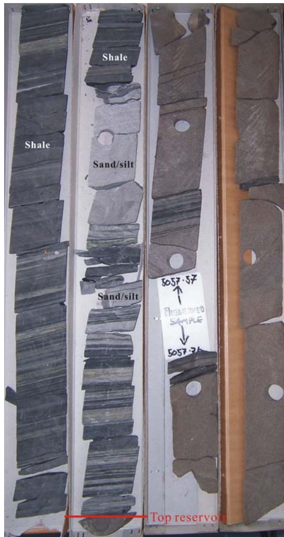
Figure 2.8 Photograph of drill core of interval 5056-5059 m (driller's depth), well 16/8b-A2, the Miller Field. The top of the Brae Formation (reservoir section) is marked. The Kimmeridge Clay Formation overlying the Brae Formation sandstone mainly consists of shale-sand/silt alternations, so called 'tiger stripe' facies.
