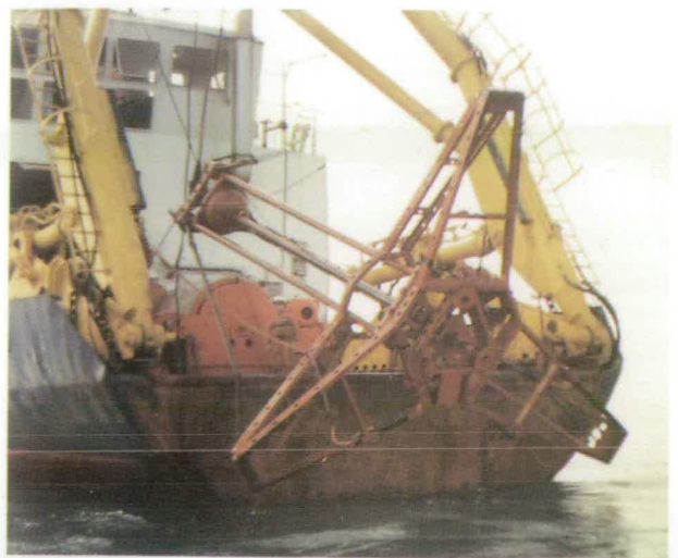
Figure 2 Deployment of the BGS 6-metre vibrocorer over the stern of the sampling vessel. The equipment weighs approximately four tons and can be operated in water depths down to 2000 m
