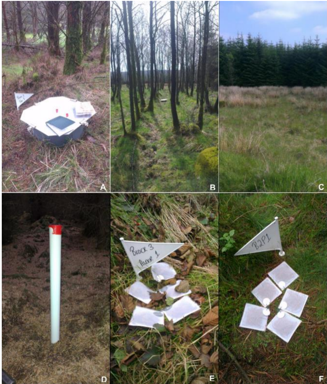
Figure 3.2. Examples of plots and set-up at Gisburn Forest Experimental site. (A) Static chamber on a planting ridge in the Scots pine plot in Block 3, (B) Static opaque chamber in a trough of the common alder plot in Block 3, (C) Block 1 grassland with Sitka spruce plot in the background, (D) Water table dipwell in the Sitka spruce plot in Block 2; also shows lack of understory cover and dense litter cover, (E) Freshly placed litter bags in Block 3 common alder plot; also shows understory and litter cover, and (F) Litter bags in Block 2 Scots pine; also indicating grassy understory and pine needle cover. All images taken by Kim Parmar, 2013/2014.
