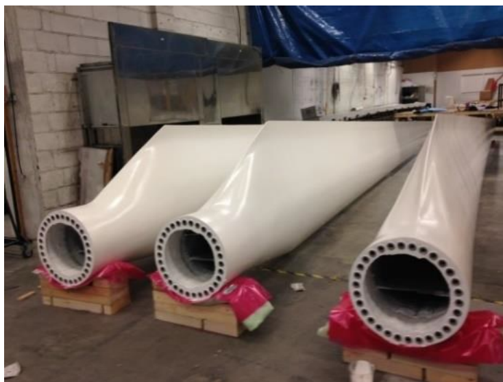
Figure 1.7. 12.6 m long wind turbine blades made using epoxy powder.
