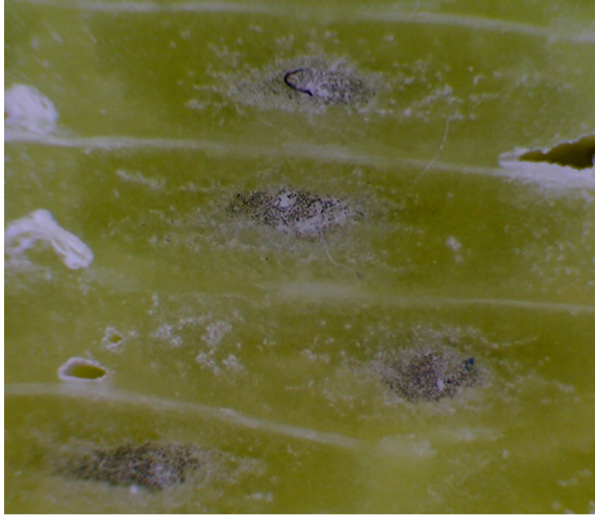
Figure 6.14. USB microscope image of the upper third of Test Laminate 1 (X1 magnification). Both incomplete tow impregnation and inter-tow voids are visible.
