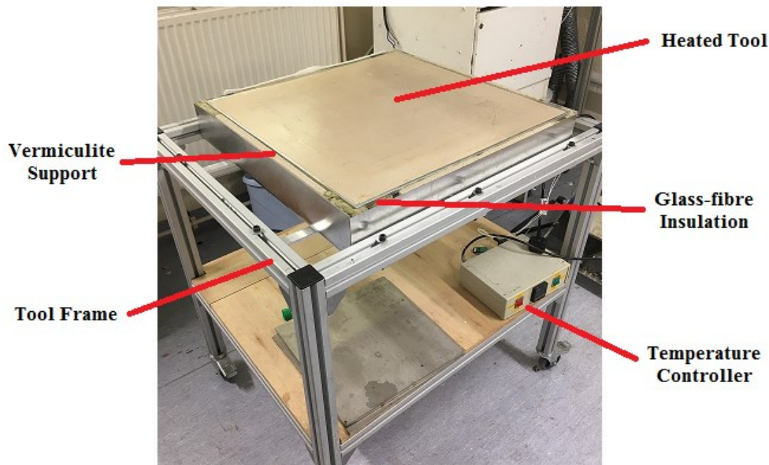
Figure 6.2. Photo of the modified heated tool and tool frame.
