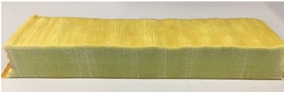
Figure 6.13. Cut-section of Test Laminate 1 showing the non-uniformity of thickness.
