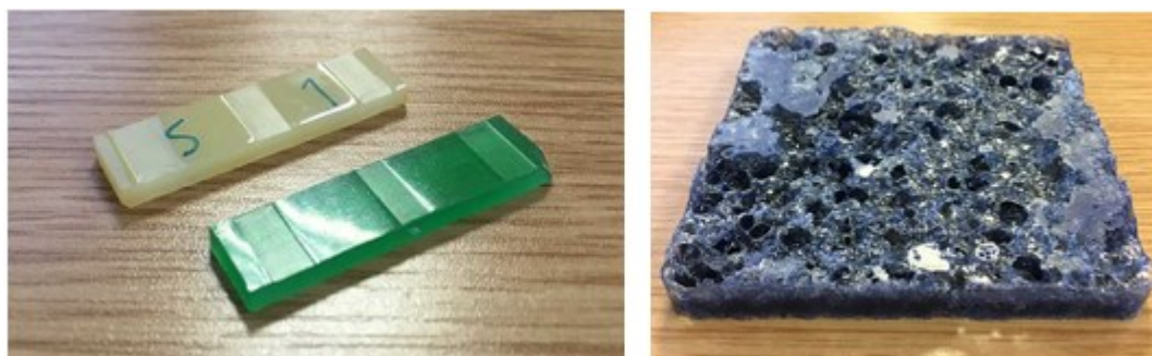
Figure A.8. Images of DMTA test specimens: (L) GRN 918 (yellow) and Ampreg 22 (green); (R) A-S-SET 02 suffered from severe porosity after being processed under vacuum.
