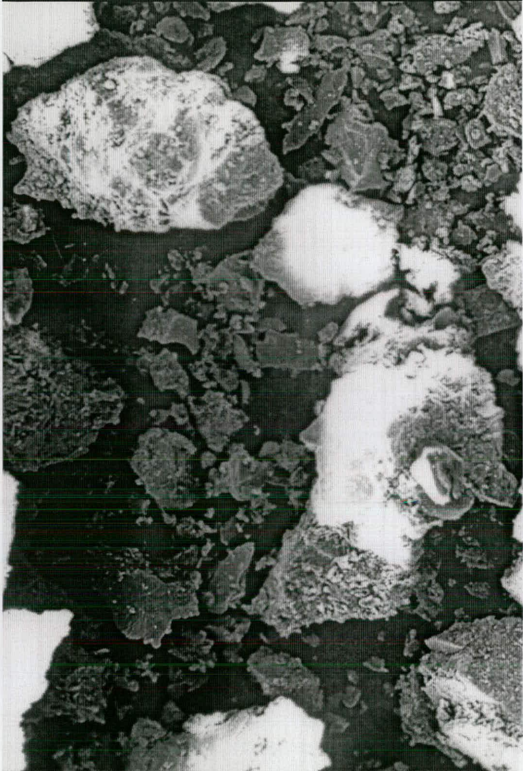
Figure 4.18 A Scanning Electron Microscope image of a disaggregated sample from one of the Penguin cores. Note that the discrete larger grains in the image are intact sand grains complete with diagenetically altered surfaces. Fine silt and clay particles are also present and generally display the angular, euhedral morphologies expected of cement crystals. These morphologies indicate that the disaggregation technique has not significantly damaged or powdered the delicate crystals present. The result is likely to be adequately clean, low-contamination illite aliquots.
