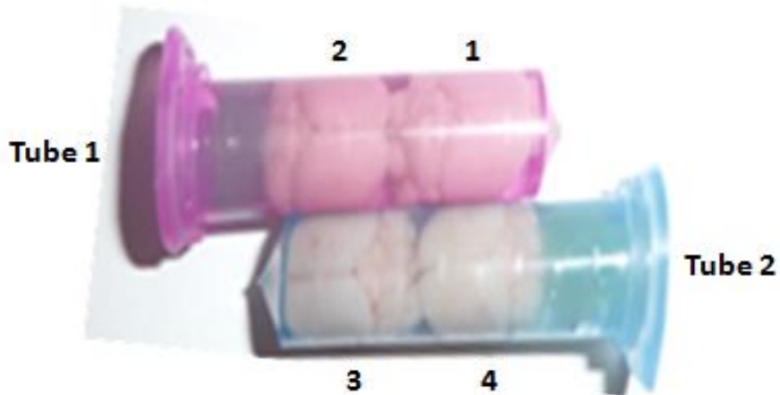
Figure 2.8.: Brains set up for ex vivo MRI- DTI procedure
