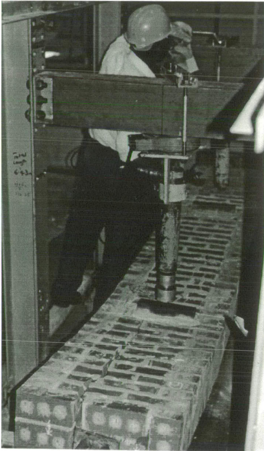
Fig 4.5-37 : Longitudinal shear cracks accompanying shear failure
