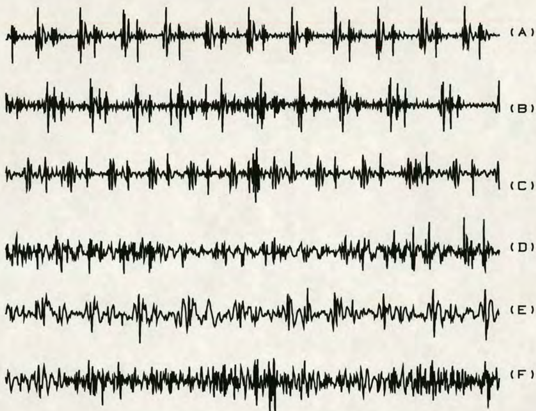
Figure 4.3 Six records, each of five seconds duration, of fetal phono signals showing a typical spread of heart pulse wave signal qualities. These are arranged from best to worst signal qualities (top trace to bottom). The respective \phi values for the traces are: \phi(A)=1.40 , \phi(B)=1.29 , \phi(C)=1.19 , \phi(D)=0.99 , \phi(E)=0.89 and \phi(F)=0.84 .
