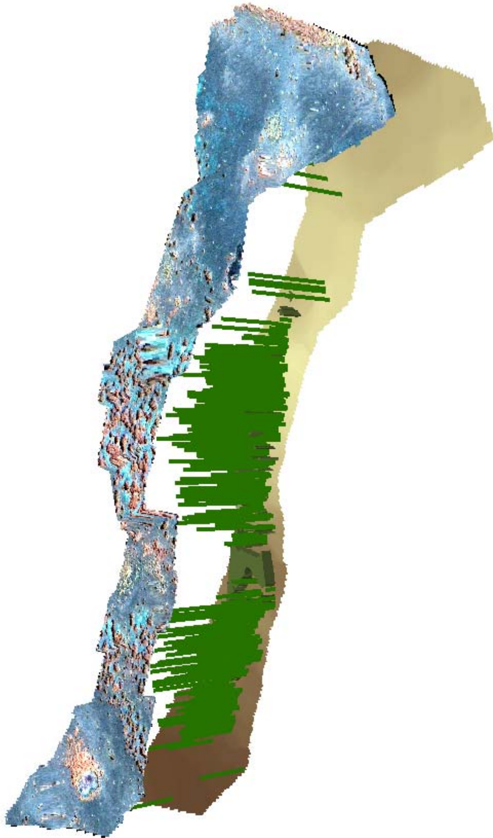
Figure 6.3: Three-dimensional figure showing the IKONOS image (4-2-3, RGB) draped on the SRTM C-band DSM. Tree heights are shown as vertical green lines and average palmetto clump heights are shown in dark green polygons. The ground surface DEM is shown in brown.
