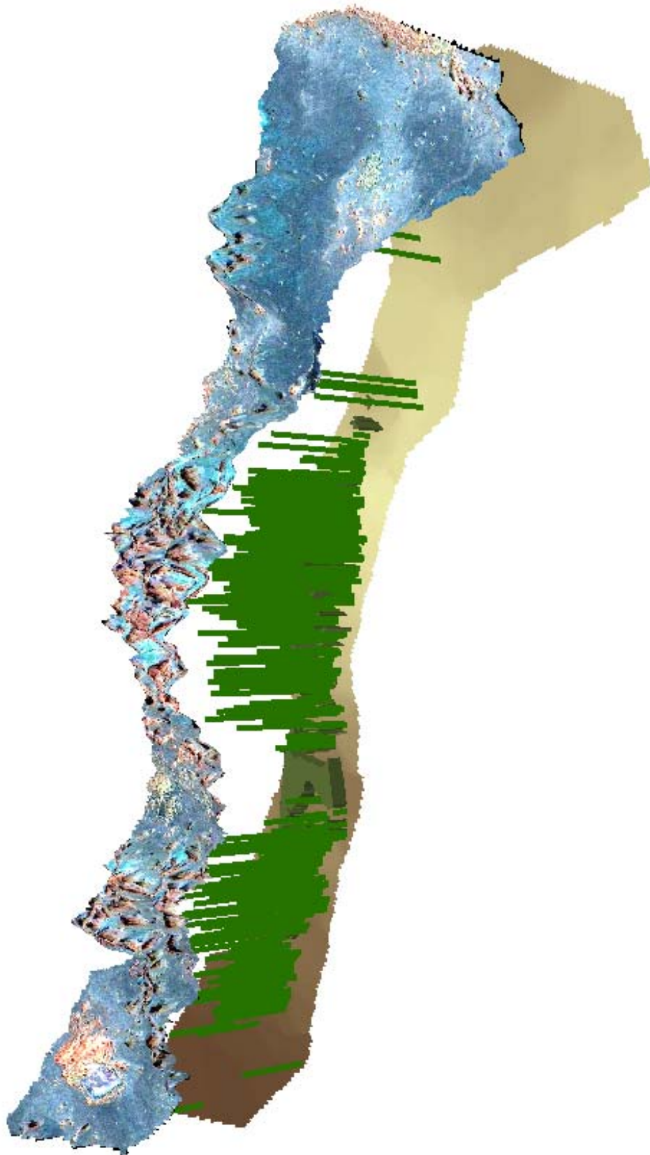
Figure 6.2: Three-dimensional figure showing the IKONOS image (4-2-3, RGB) draped on the AIRSAR C-band DSM. Tree heights are shown as vertical green lines and average palmetto clump heights are shown in dark green polygons. The ground surface DEM is shown in brown.
