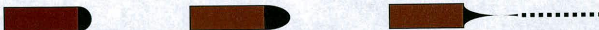
Figure 2: Effect of ESI potential on the drop at the tip of the capillary with increasing voltage. (left) At low voltage, the drop is almost spherical. (Centre) At about 1 or 2 kV but below the onset potential the drop elongates under the pressure of the charge accumulating at the tip. (Right) At onset voltage, the pressure is higher than the surface tension, the shape of the drop changes at once to a Taylor cone and small droplets are released. The droplets divide, producing spray.
