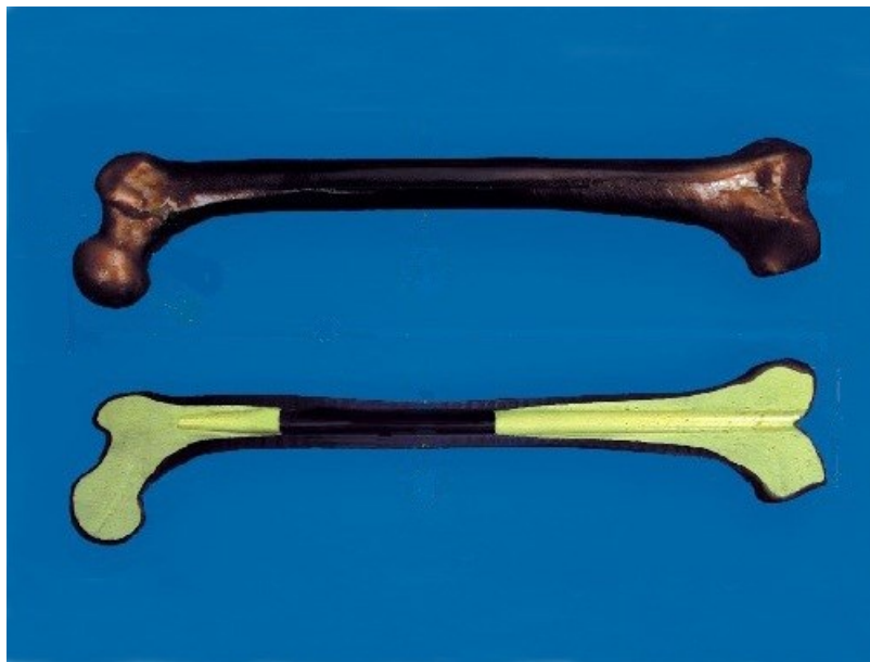
Figure 8.8: Image showing external (top) and internal (bottom) cortical and cancellous bone regions of the fourth generation composite femur, image adapted from ( http://www.sawbones.com/products/product.aspx?1937 ), retrieved 02/12/2008.
