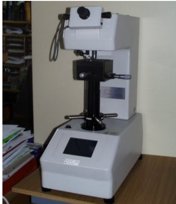
Figure 3.3.2.2: Microhardness tester fitted with a Knoop indenter as used for microhardness testing of donkey and horse teeth.
