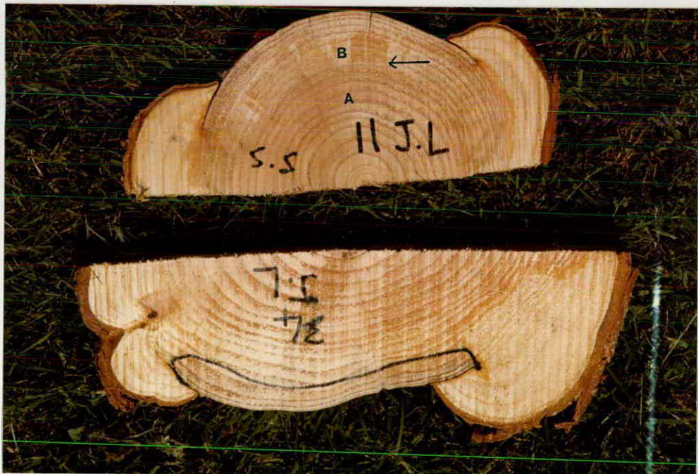
Plate 10: A cross section in a Japanese larch which was infected with S.sanguinolentum entering through extraction wounds A. Clear heartwood B. Infected wood
