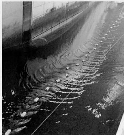
(c) MEM-based floating ribbon in GWK, Hannover Flume.
