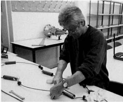
(a) Preparing the 18m GWK sensor - insertion and wiring of moulded sensors
