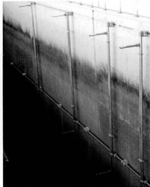
(b) Image of GWK facility, Hannover showing resistance wire wave gauges
