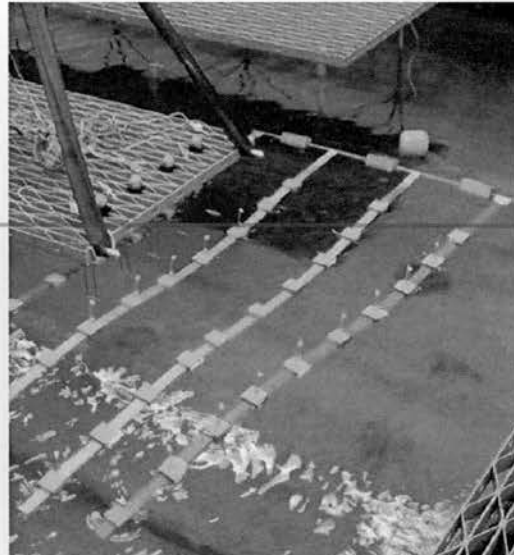
(b) Inactive floating ribbon (as array) in Edinburgh Curved Tank
