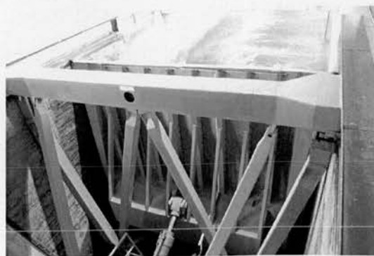
(c) The 307m, 800kW GWK Flume, piston type wave maker
