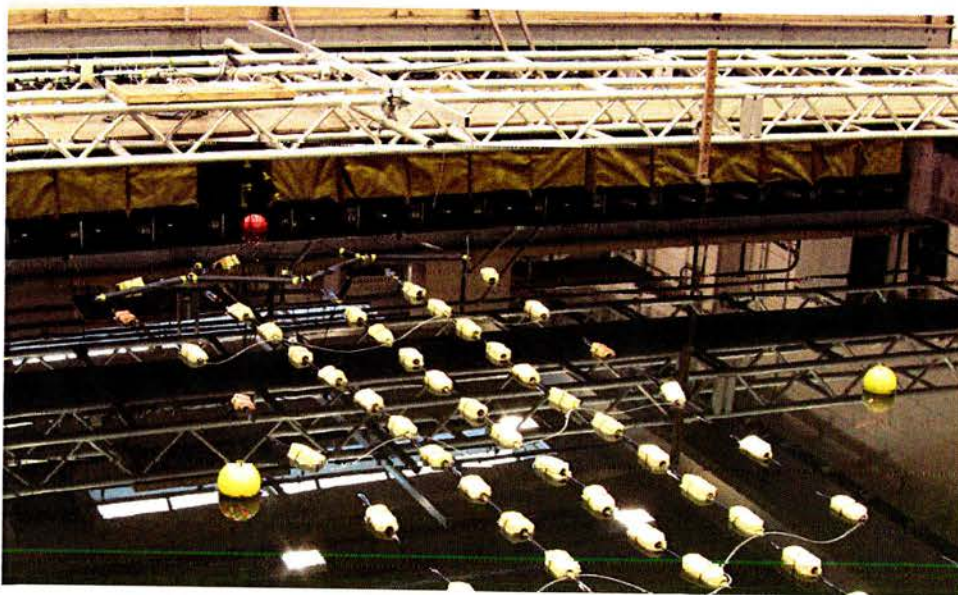
Figure 6.27. Paddle failure ends testing. Spring failure on paddle number 7 (4 from left in image).
