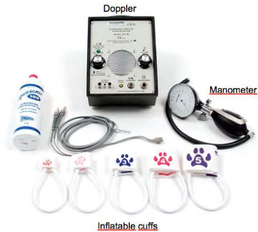
Figure 17. Material used for systemic arterial blood pressure measurement using the Doppler method. Source: www.dispomed.com
