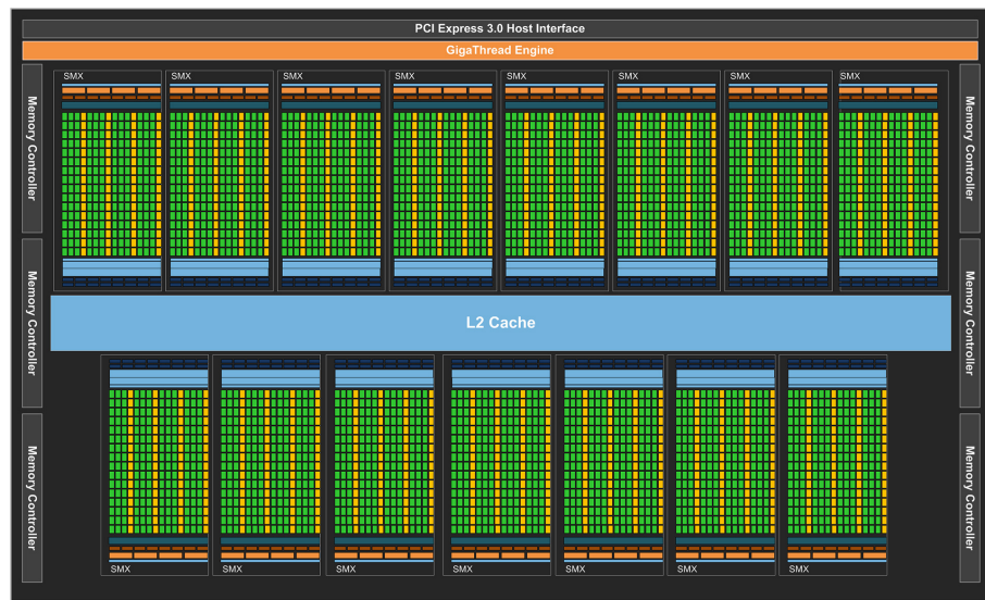
Figure 1.2: Block diagram of the Kepler K40m GPU.
