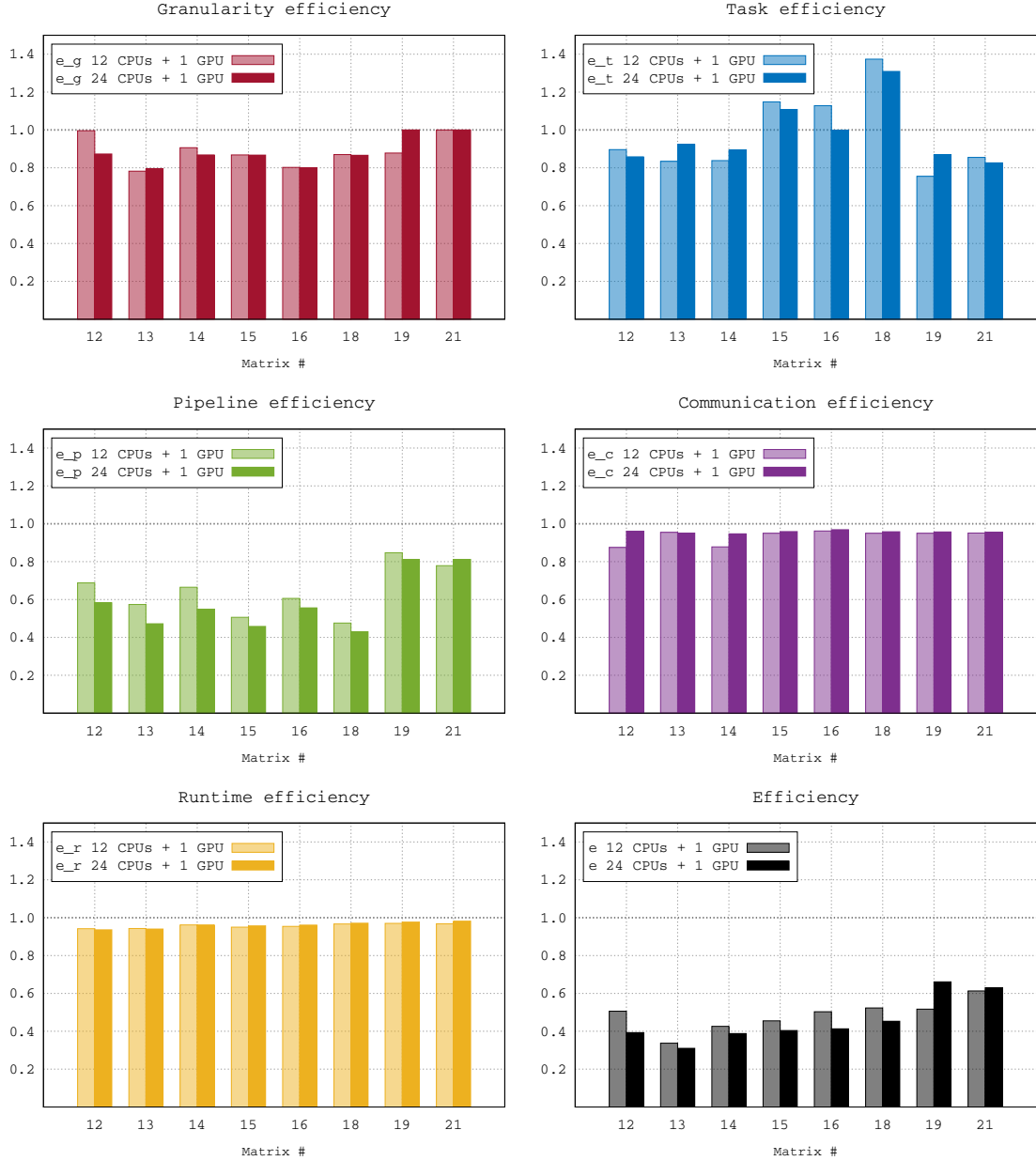
Figure 6.8: Efficiency measures for the STF heterogeneous algorithm on Sirocco with both configurations 12 CPUs (1×E5-2680) + 1 GPU (1×K40M) and 24 CPUs (2×E5-2680) + 1 GPU (1×K40M). Note that due to technical issues in StarPU, we are currently unable to obtain the efficiency measures for matrix # 17.
