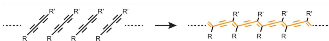
Figure 2.11 Polymerization reaction of diacetylene compounds from ref. 18 .
