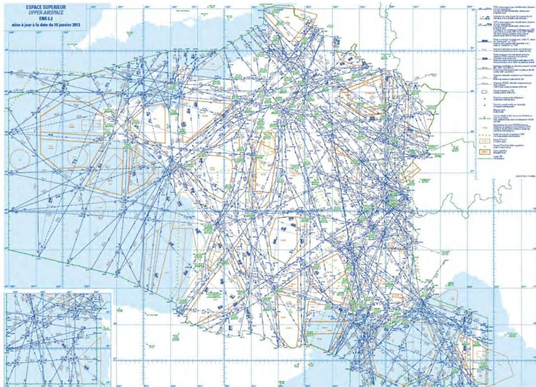
Figure 1.1: Airways (represented by blue lines) and way-points (intersecting points) over France for the upper flight information region (above FL195). Credits: SIA
