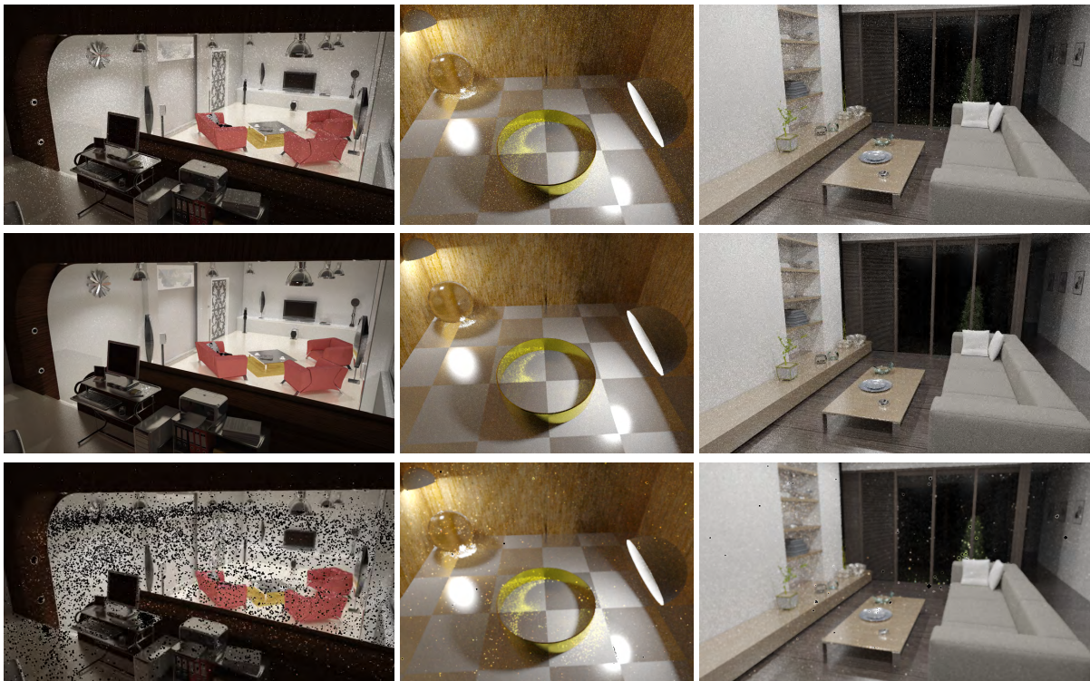
Figure 7.3: Results of our method, and comparison with Xu et al. method. First row: original HDR images. Second row: after despeckling by our method. Third row: Results obtained by Xu et al. method, with a window size of 4 and a range factor set to 0.01.
