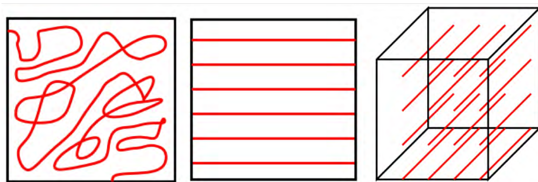
Figure 8: [98] Example of acquisition trajectories for mobile sensing in 2D and 3D settings.
