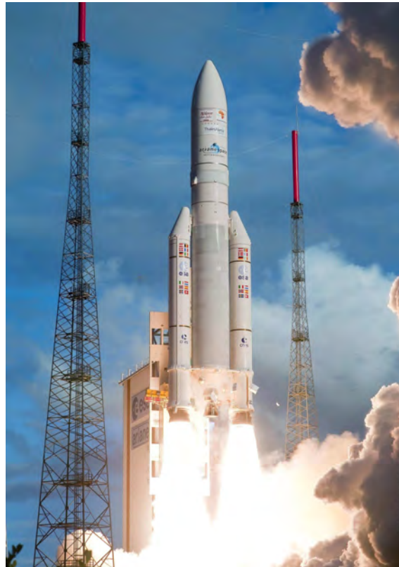
Figure 1.3 – Lift-off of an Ariane 5 ECA launcher (launch no. 196) from Kourou, French Guiana. During this phase, the two boosters provide 92% of the total thrust.
