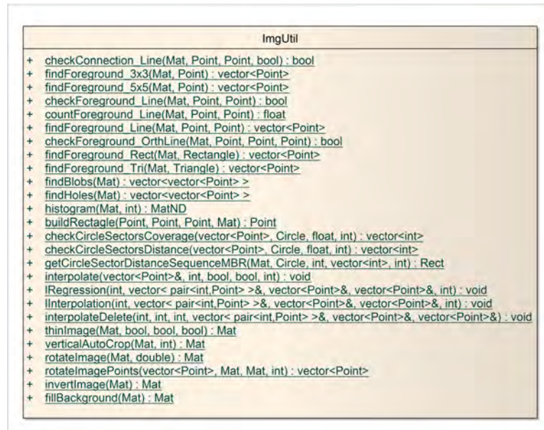
Figure 6.4: Class diagram of the util package: image utility library.
