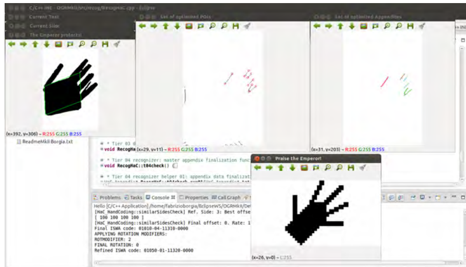
Figure 6.37: Screenshot representing the completed recognition of a glyph belonging to the Hands Configurations area.
