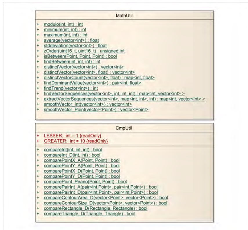
Figure 6.6: Class diagram of the util package: math utility library and comparison library.
