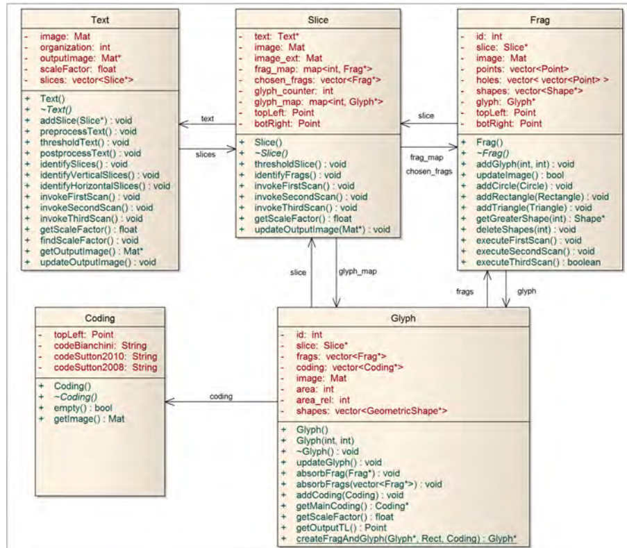
Figure 6.3: Class diagram of the beans package.
