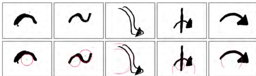
Figure 6.18: Application of the generalized Hough transform for the detection of curves to images which do not contain circles.
