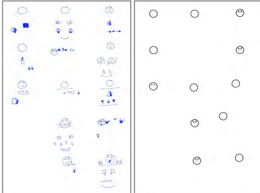
Figure 7.3: A handwritten page belonging to the DS-TEST-POITIERS dataset, as it appears before (left) and after (right) the recognition of the glyphs belonging to the Facial Expression: Eyes area.
