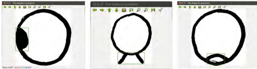
Figure 6.25: Feature recognition applied to a set of glyphs belonging to the Head Circle and Contacts area.
