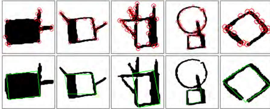
Figure 6.20: Polygon detection algorithm implemented within the SW-OGR Engine, applied to glyphs featuring rectangular shapes. The algorithm uses the Shi and Tomasi method to locate the corners in each image (top). Afterwards, the corners are processed in order to build the polygon, if this is possible (bottom).
